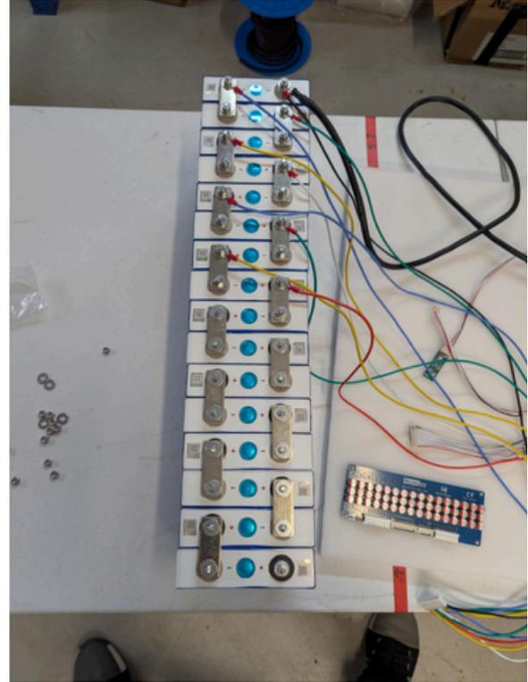
*Note: Ensure that you use the correct order as getting this wrong could result in damaging the balancer and/or the BMS.*
