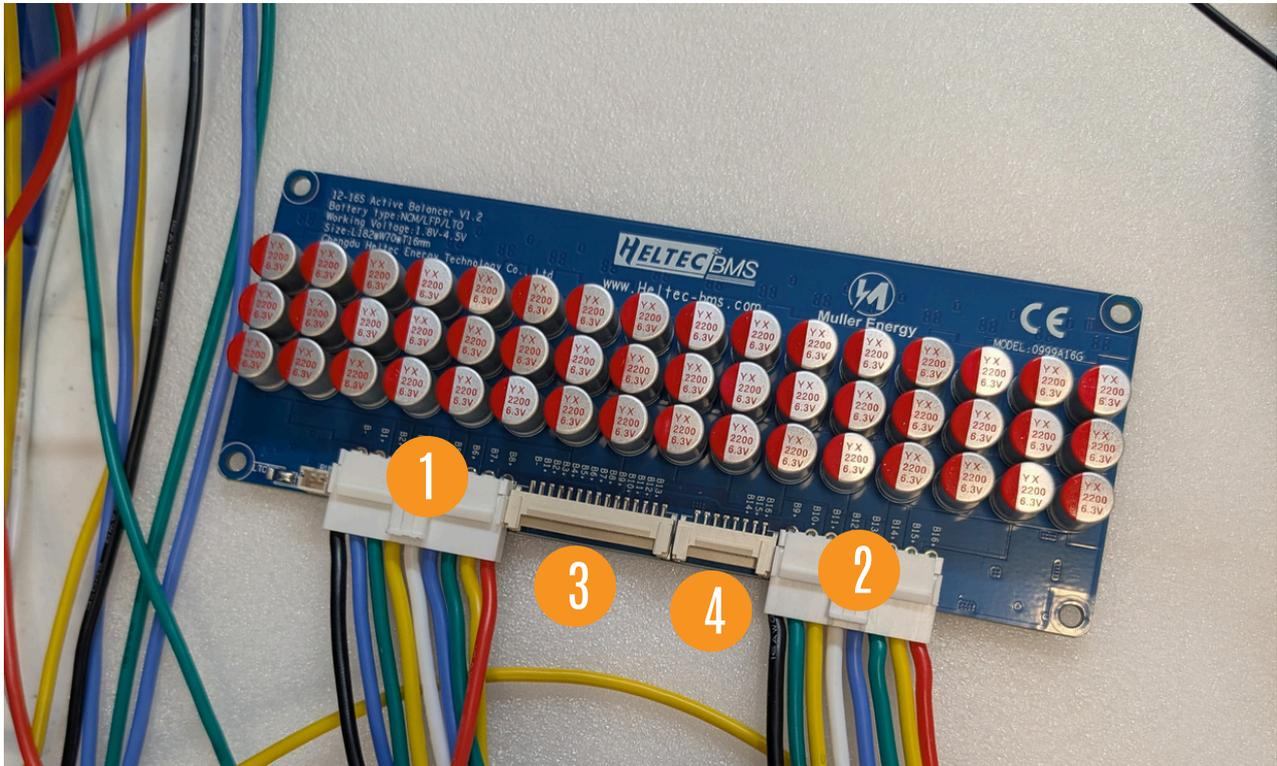
**8.** Locate the balance wire. It will plug into the BMS where it says "Balancer" and in the 2 pin connector on the active balancer.
