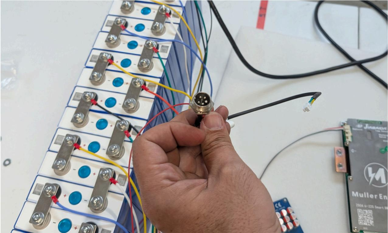
Then take the black cable on it and connect it to the main negative terminal. You can now tighten the nut. Do the same with the red cable. Then take the two pin connector and plug it into the BMS where it's labelled "RS485".
