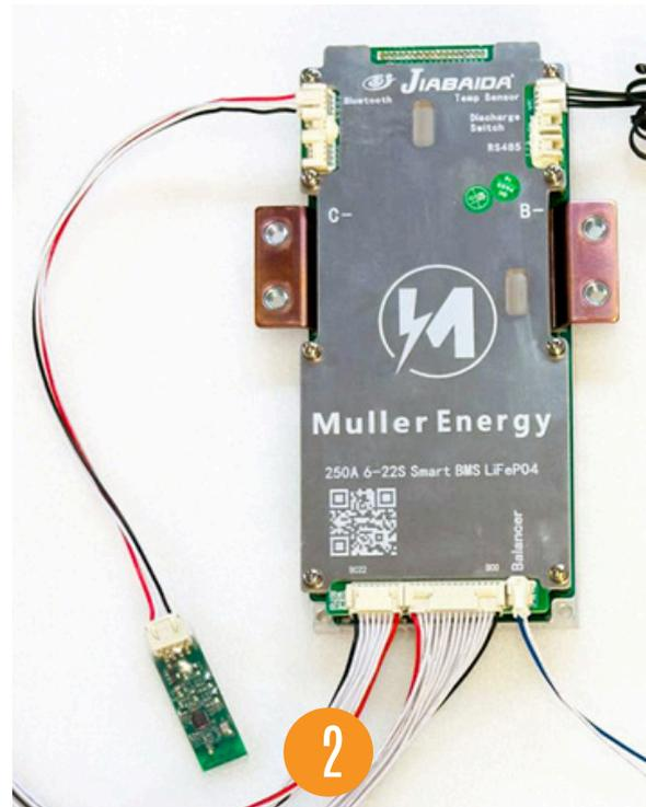
*Optional: Connect the connector with the two open ended cables to the socket called "Discharge Switch"*
